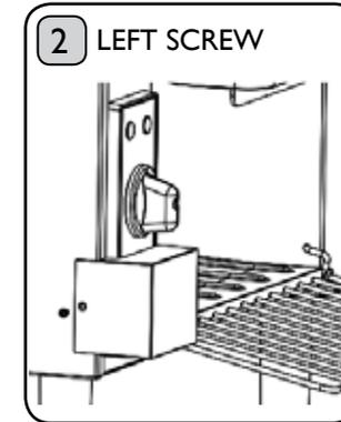
Insert and tighten the left-hand screw.
