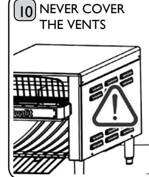
Never cover the vents on the sides of the DCT2i. This will prevent necessary air flow and could cause a fire.
