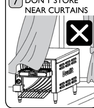
Do not store or use your DCT2i next to curtains or flammable material. **A fire may occur if incorrectly positioned.**
